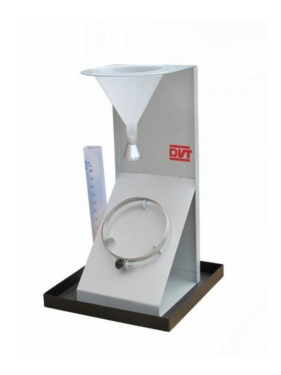
USED IN THE DETERMINATION OF WATER RETENTION OF TEXTILE SURFACES
